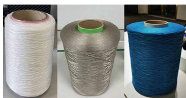
抗污聚酰胺 6BCF 原色丝及有色丝 Primary color yarn and colored yarn of the Anti-fouling Polyamide 6 BCF
